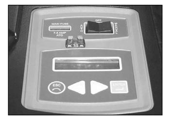
Figure 22. Remove 7.5 Amp Fuse
